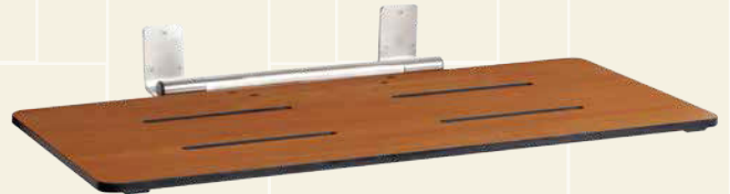
REAR MOUNT TUB SEAT This seat top attaches to the rear of the tub and conveniently folds up against wall to save space. Supported by a #304 solid stainless steel frame. Shown here in 1-piece phenolic teak. WIDTH: 29" | DEPTH: 16.5
